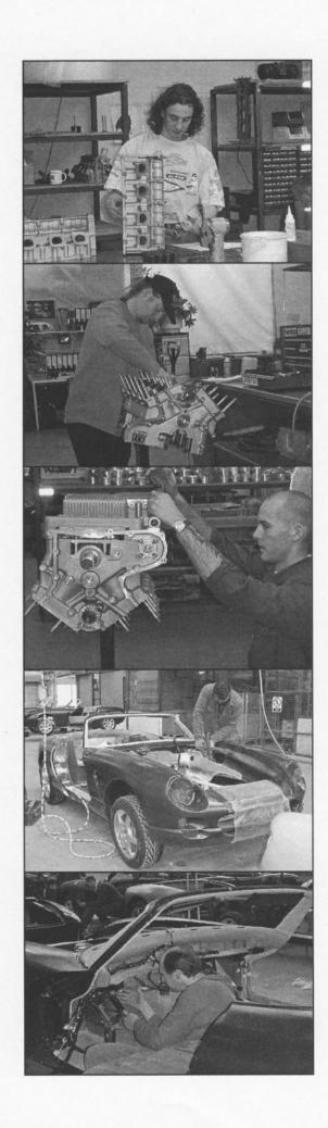
The Griffith 500 and Chimaera are powered by TVR modified Rover based V8 engines. Work on these engines is carried out at the sister company, TVR Power in Coventry. The completed units in 4.5 and 5.0 litre form are transported to Blackpool ready to be fitted to the cars on the assembly line.
