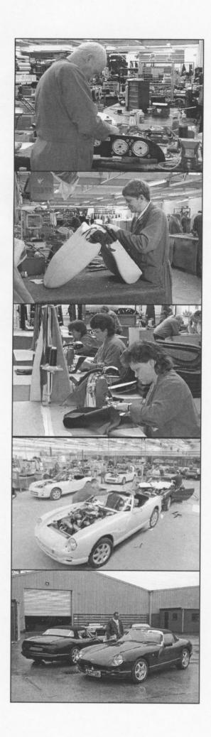
Stage 4 - The trim shop prepares all carpets, trim and dashboard prior to installation. This involves cutting and sewing carpets, leathers, vinyls and mohair (for the convertible's hoods) to exacting standards. These are then fitted to the car. Because of the uniqueness of each car, this work is done to order rather than for stock.
