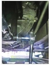
I should point out that fitting is not as easy as it would first seem, as the magnet wants to stick to everything, including the hole where the plug goes and the sump itself! The best way I found of getting it in and lined up was to use an Allen key socket.
