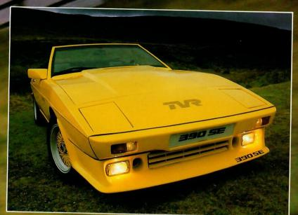
Power comes from the 3.9 litre, 275 BHP fuel injected V8 engine. Handling derives from the uprated chassis and continuous drive differential. Braking is by ventilated discs, large calipers and balance system.
