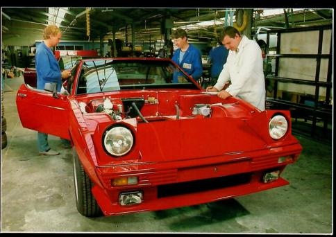
An almost complete car receives its hood installation along with one of the numerous quality control checks nearing the end of build. When
