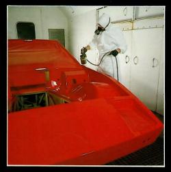
In due course the painter will take almost a day to carefully layer on the many coats of paint required to achieve the mirror like finish of the final production car.
