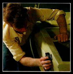
Meticulous care and attention to detail at the priming stage will ensure perfect finish later on. Rubbing down by hand between each of the five coats prepares the surface for the application of the paint.
