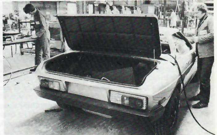
Cars are water tested using a hosepipe!
