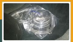
The speaker was then free and immediately put into a plastic bag as the speaker is a large magnet which will pick up any metal when it is put down. Any metal picked up has the potential to damage the delicate parts of the speaker.
