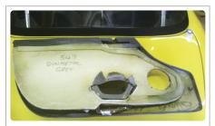
Once the carpeted bit has been removed you will come across a clear plastic sheet which is lightly glued around the edges and covers the aperture in the door. With a little persuasion this can be pulled, intact, from the door.
