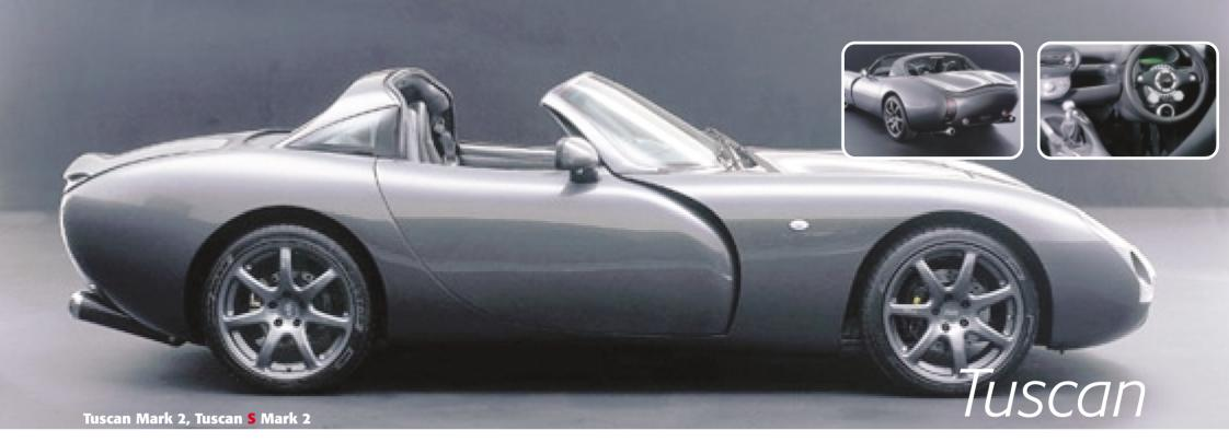
2 seater with removable roof panel and rear window or Straight 6 engine with rear wheel drive
