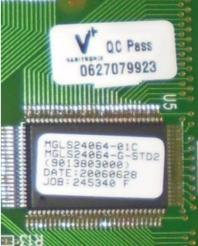
Re-fit and re-connect the new LCD module. As it is 5 mm thinner than the original, the spacer bolts need to be replaced also (I needed to carefully cut one in place using a Dremel because I couldn't remove it).
