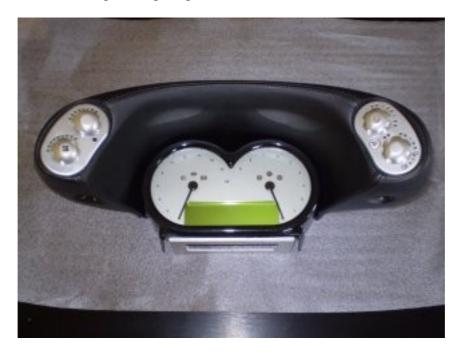
The complete dash back in the T350. Different display colour, but no more missing lines:
