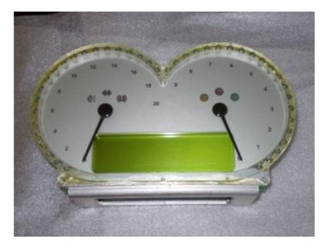
Re-attach the POD cover using a hot glue gun and fit it back to the dash:
