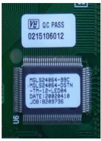
The replacement LCD module is also from Varitronix: MGLS24064-01C (MGLS24064-G-STD2). The connectors (Tyco Electronics / AMP: 20 way straight header + 3 way connector) need to be soldered into the new module:
