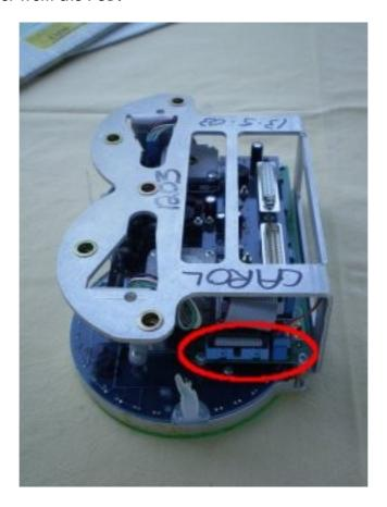
Disconnect the ribbon (data) cable and back-light cable. Remove the four screws holding the LCD module:
