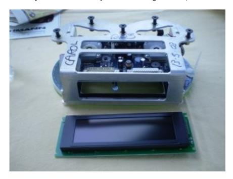
The LCD module is a Varitronix MGLS24064-99C (MGLS24064-DSTN-TM-12-LED04):
