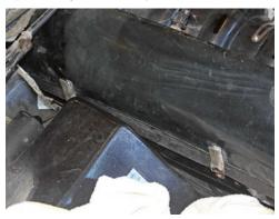
are on the outside edge of the air-box and hold the top to the bottom. These normally have a split pin through them to stop them coming undone accidentally. The third is on the inside, about halfway along the back between the air-box and the engine. This is a James Herriot moment and requires your hand going between the two. On my car it is possible to do this with the engine at operating temperature as long as you are careful.
