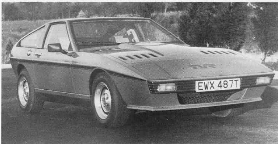
Above, an aggressive front end with integral spoiler and flip-up headlamps.
