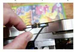
If you have a Code A or B then the micro switch that you want to get to is behind the gold plate with the speed markings on it. On mine this was just lightly glued on and just lifted off with a little light persuasion (fingers only). The glue was only just enough to hold it in place as you mount the pod, as the speedo plate is actually held in place anyway when you put it all back together.
