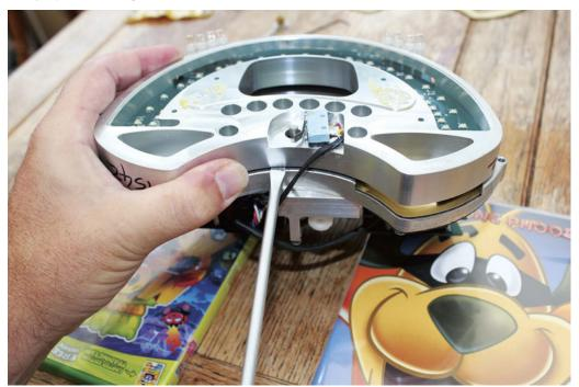
As it was my temperature gauge that had the problem, I had to separate the two metal bits of the pod. These are not actually secured together with screws, but held in place via two roll pins, and I used a flat bladed screwdriver to slowly and gently prise the two parts apart. This was a little unnerving the first time I did it. When the two halves came apart I had to disconnect the two ribbon cables that connect between the backlight circuit board and the rest of the circuitry.
