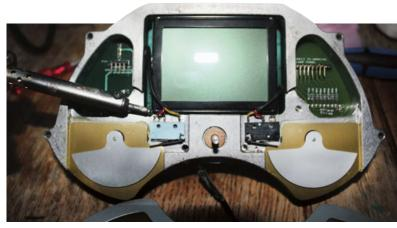
Fitting the switch is a case of soldering the two wires on, then pressing the switch onto the fittings, which I easily achieved by pressing it with my fingers. I did have to lift the lever when fitting the switch so that it cleared the back of the temperature gauge.
