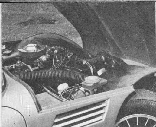
Forward hinging bonnet reveals all—but could tip further to give more headroom. Note the very accessible battery and small Weber air cleaner
