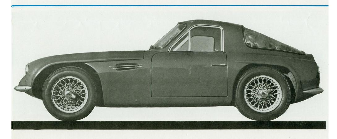
**Technical Specification** Manufacturer: British Motor Corporation. Type: Four stroke OHV. Cylinders: 4 in Line. Bore: 3.16 in. (80.26 mm). Stroke 3.50 in. (89.00 mm). Capacity 109.6 cu.in.(1798 cc). Compression ratio:8.8-1. B.H.P: 98 @ 5400 r.p.m. Torque: 110 Ft. lb. @ 3000 r.p.m. Transmission: 4 speed. Fuel: Premium. Electrical System:12v. Type of Carburettor: Twin SU H S 4 1½ in. Clutch: Borg and Beck 8 in. Diaphragm spring, Hydraulic operation.
