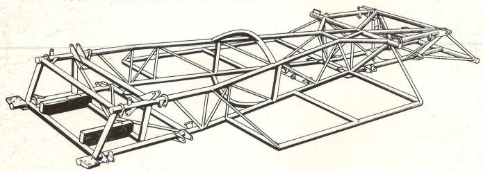
Along with many other technical advances the Mark III 1800 possesses a backbone structure second-to-none, and this has been race proven time and again. Offering enormous strength and torsional rigidity yet with an unbelievable lightness, this multitubular frame provides an unparalleled handling quality and safety margin for both driver and passenger, even under the most severe conditions.
