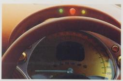
gear change lights green @ 6000 rpm amber @ 6500 rpm red @ 7000 rpm
