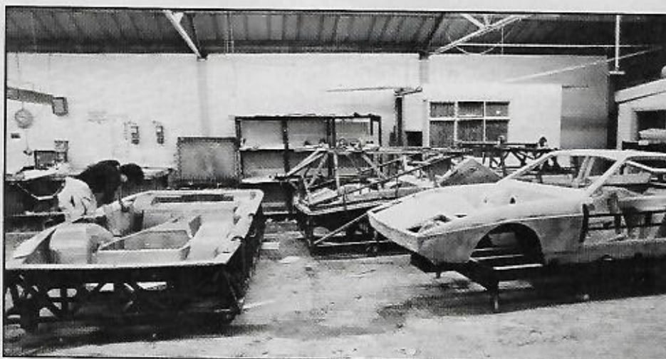
Work starts by laying up the glassfibre in a base mould, while top and bottom sections are clamped together in moulds just behind completed body shell.
