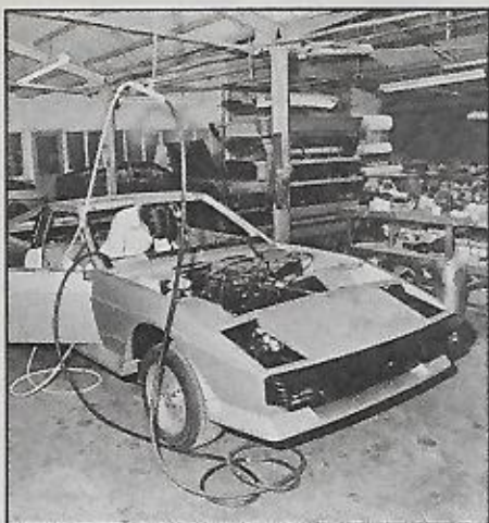
Looking more like a car now, a Coupe gets its seats and interior trim.
